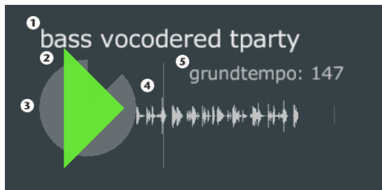
Figure 2: The loop component (zoomed in), (1) the caption, (2) play/stop button and indicator triangle, (3) pie diagram animation of loop progress, (4) loop waveform and progress indicator (thin vertical line), and (5) the base tempo of the loop.
