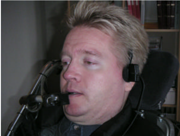
Figure 5: A user with headset and a sip-and-puff unit.
